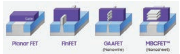
Figure 1. Evolution of transistor model and complexity (source: Samsung)
