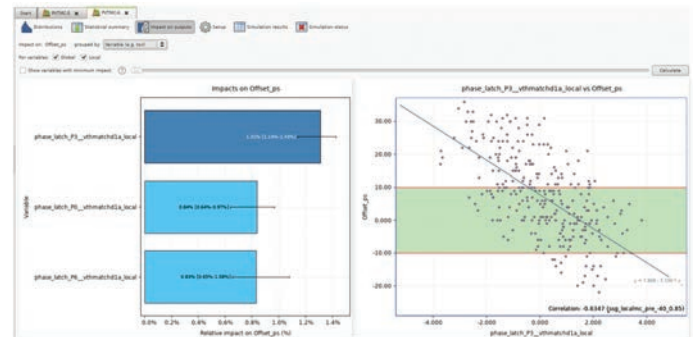
Figure 3. Comparator-Latch sensitivity analysis results.
