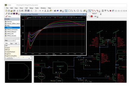
S-Edit schematic capture and simulation cockpit shows schematics, simulation waveforms, model parameters and simulation settings. The tool is easy to use and has the power to handle complex mixed-signal IC design capture.
