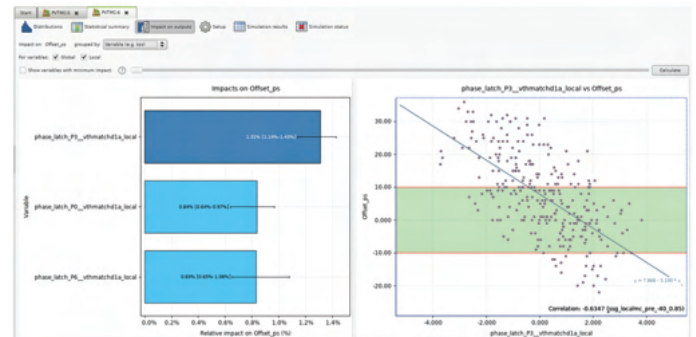
Figure 3. Comparator-Latch sensitivity analysis results.
