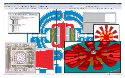
A central part of the MEMS design flow, here Tanner L-Edit MEMS is shown being used to design a magnetic actuator; the tool allows for the quick creation of entire complex curved shapes for MEMS from just a few easily drawn shapes.
