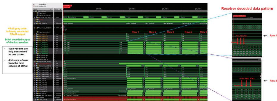
Figure 12: Top level digital simulation results (full-chain mixed-signal sim using row injection).
