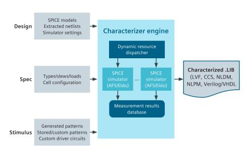
Kronos Characterizer is a high-performance, high-throughput, general purpose cell library characterization tool for standard, multi-bit, and I/O cells.
