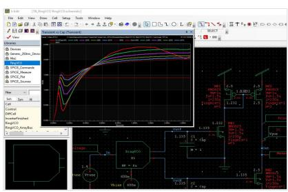
Tanner S-Edit schematic capture and simulation cockpit shows schematics, simulation waveforms, model parameters, and simulation settings. The tool is easy to use and has the power to handle complex mixed-signal IC design capture.
