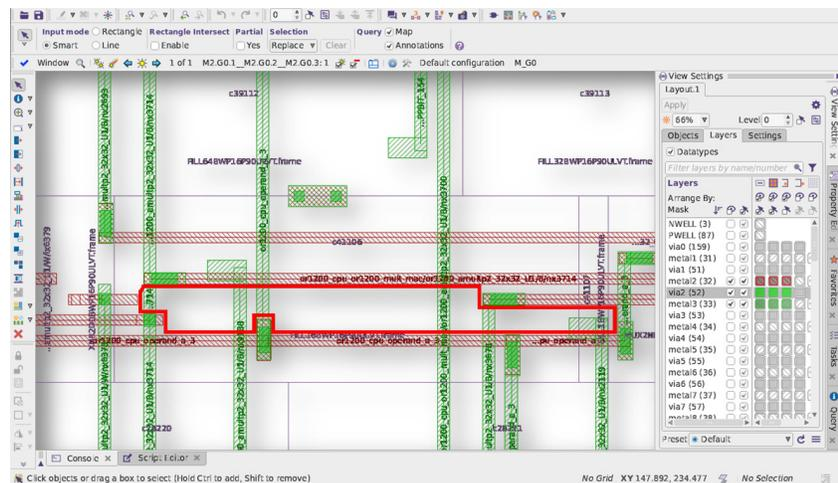
The Calibre RealTime Digital platform completely changes the traditional digital design DRC closure flow by bringing Calibre sign-off quality verification into the P&R environment.
