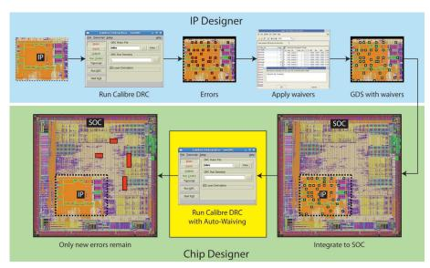
Calibre automated waiver management ensures IP quality while eliminating redundant error debugging and waiver negotiations during IP integration.
