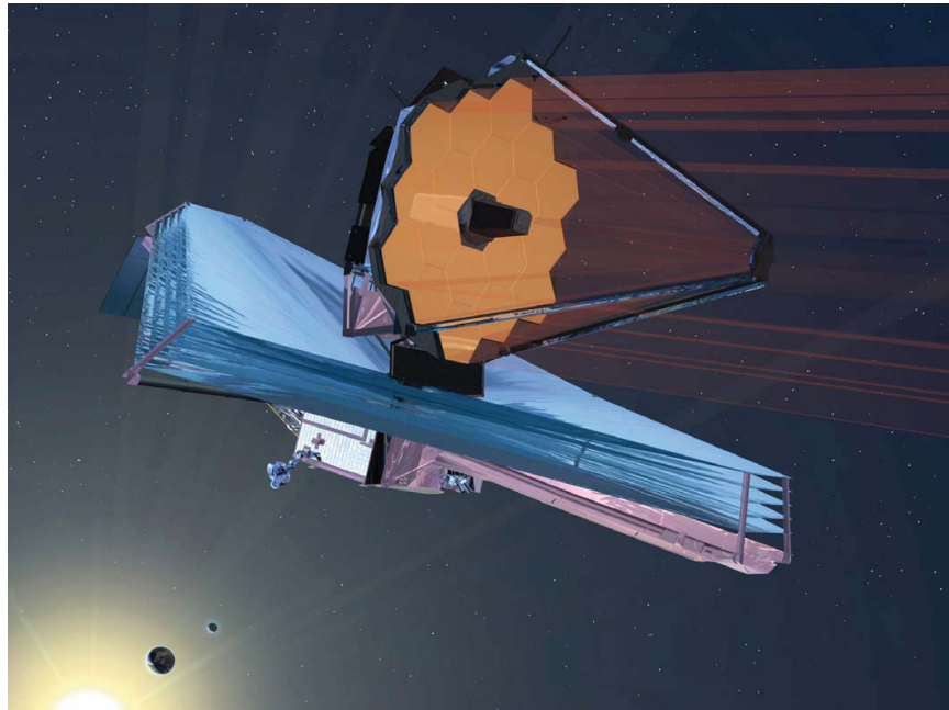
Figure 2: an artist's impression of the deployed JWST in L2 orbit showing the 6.55 m segmented telescope mirror and matching sunshade (Source: Northrop-Grumman).
